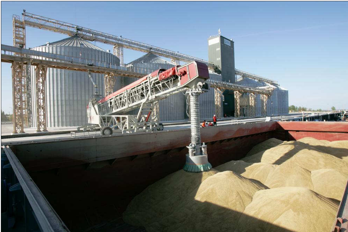
Figure Four - Integrated Telescopic Chute and Dust Covers eliminate dust emissions during loading cycle
